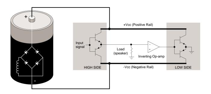
Figure 2. Crown Patented Grounded Bridge Topology
